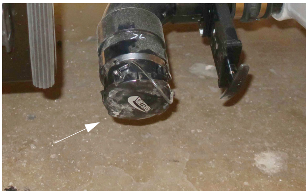
Sewage Drain Outlet/Dust Cap (Located in driver side compartment) -Typical View
