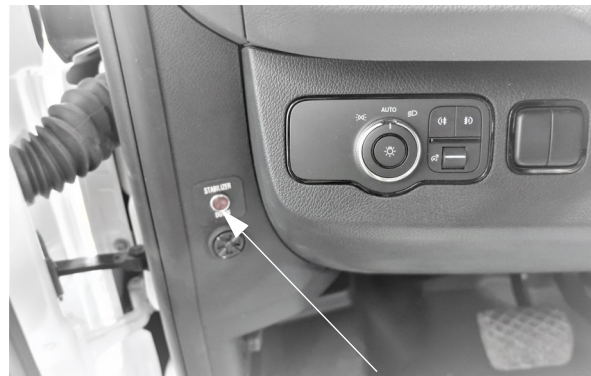
“Stabilizer Down” Light (Located on driver side dash) -Typical View
